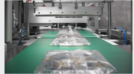
Guillotine-type or box-motion cross sealing system
